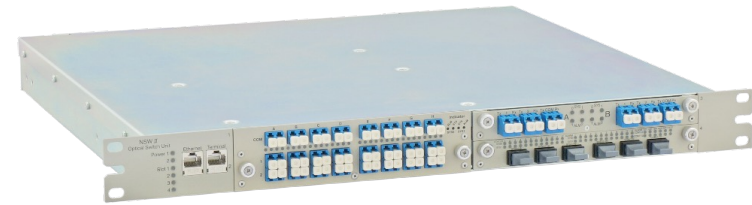
Physical layer switching device (Intelligent optical switch)
