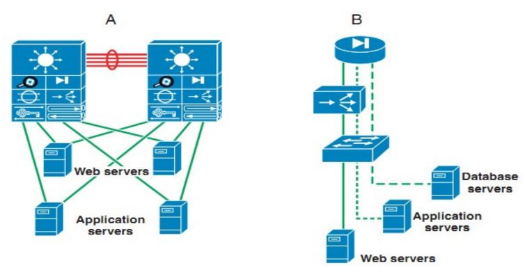
Physical segregation improves performance because each tier of servers is connected to dedicated Hardware. The advantage of using logical segregation with VLANs is the reduced complexity of the Server farm. The choice of physical segregation or logical segregation depends on your specific network performance requirements and traffic patterns.
