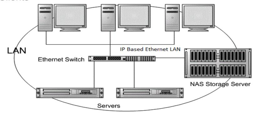
NAS is storage that is connected directly to a network, such as a LAN, that provides file-level access to data using standard protocols such as NFS (Network File System) or CIFS (Common Internet File System).
