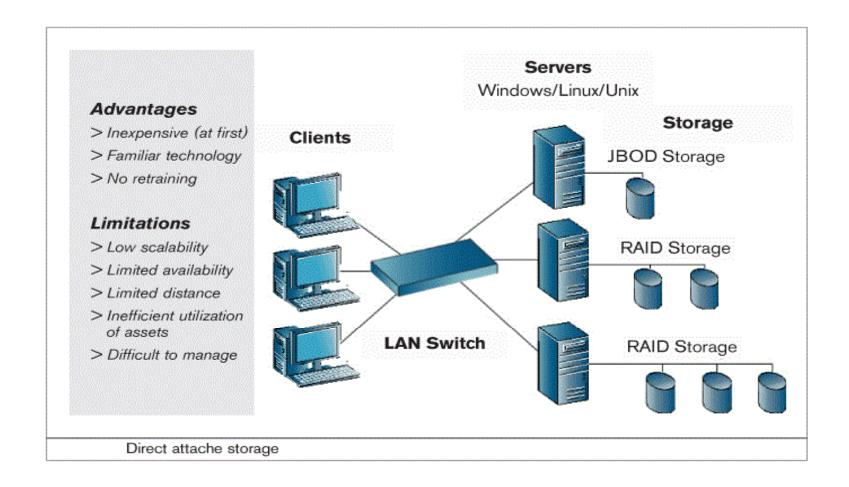
DAS means each server has dedicated storage that is directly connected to that device. The storage device is seen and accessed by a single host system, and in the event that another host system will need additional storage, that host will add more physical storage and/or I/O interfaces or host bus adapters.
